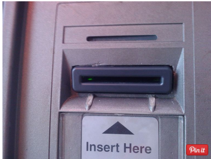
A card skimmer inserted in an ATM. Note the damaged plastic and mismatched color. ThisIsntExeter | flickr CC BY 2.0
